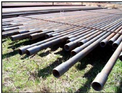
3465ft (110jts) 2-3/8in Chrome Tubing, 5.80#, Chrome L-80, w/ Mannesmann TDS Connections, R-2
